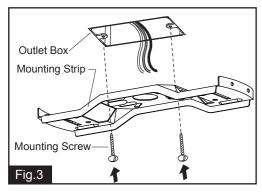
Tighten the mounting strip to the outlet box with 2 mounting screws. (To reduce the risk of fire electric shock, or personal injury, mount to the outlet box marked "Acceptable for fan support" and use mounting screws provided with the outlet box.)
