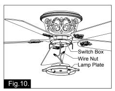
Make wire connections using wire nuts:
