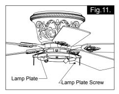
Attach the lamp plate to the switch box by aligning holes, then secure it with lamp plate screws.
