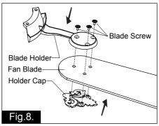
Attach the holder cap and the blade holder to the fan blade by aligning holes (the fan blade should be placed in between blade holder and blade holder cap). Then secure them with three blade screws. Repeat with the others fan blades.
