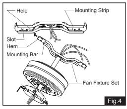
Attach fan fixture set onto mounting strip. Insert one end of mounting bar through the hole of the mounting strip, locate the hem of the mounting bar into the slot of the mounting strip. Repeat with the other end of the mounting bar.
