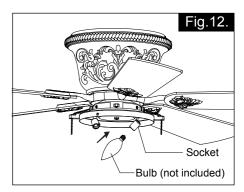
Install bulbs (not included). See relamping label at socket area or packaging for maximum allowed wattage.
