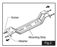
Remove the screws and washers from the two mating holes on the mounting strip. Loosen (do not remove) the screws in the mating slots on the mounting strip.
