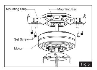
Secure the mounting bar to the mounting strip using four set screws.
