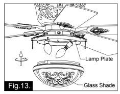
Rotate the glass shade upward to the lamp plate in clockwise.
