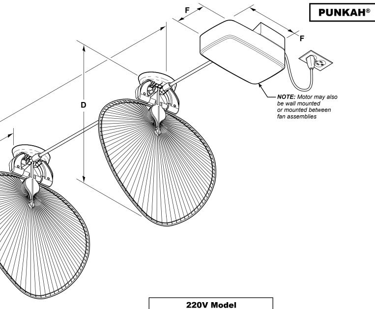
Motor Assembly - 220~240 volt, 50 Hz Ceiling / Wall Mount Oscillating RPM: 19 (single-speed) Available in 2 standard finishes
